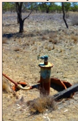
Erounghoola-1. A dry oilwell converted to an artesian water well for livestock
